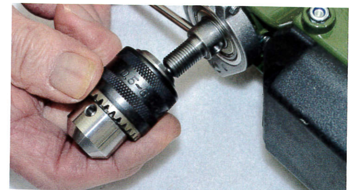
It is easy to screw the ROHM chuck to the threaded drill shank in place of the collet holder
